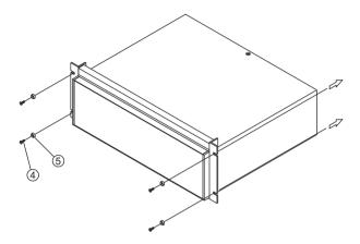
**CAUTION** The instrument may fall. Install the suitable support angles applying to the used rack system to support the instrument.
